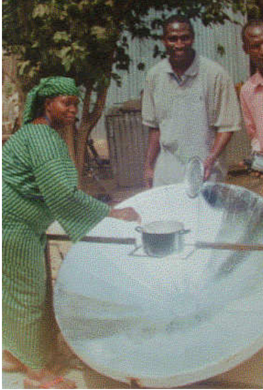
Figure 3: Parabolic Solar Cooker, BayanLoco, Nigeria (left to right: Maria Ajayi, Pastor David Adesokan, Ezekiel Kyari)
